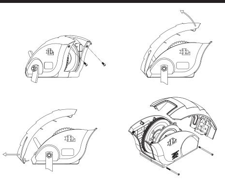
The cover comes off the winch in three pieces. To remove the top cover, loosen and remove the two screws in the front of the cover with a 1/8 hex key. Pull up on the front of the top cover and rotate the top away from the winch. Once the locking tabs are disengaged from the sides, pull the cover straight back to remove.
