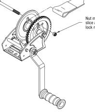
Nut must be on gear slice as shown. Use lock nut only.
