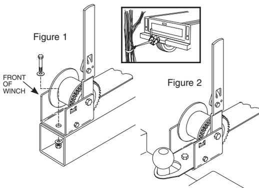
**OPERATING INSTRUCTIONS** — Wind line on winch reel by moving handle back and forth with both ratchet pawls engaged. Both ratchets should produce a loud, sharp, clicking noise.
