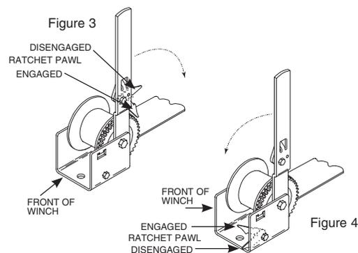
**WINCH MAINTENANCE** — This winch has been fully lubricated at the factory; but, for continued smooth performance and increased life, occasional greasing of reel shaft is recommended.
