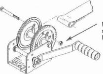
Nut must be on gear side as shown. Use lock nut only.
