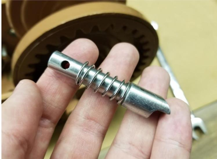
5. Grab the new ratchet plunger and spring and assemble as shown in the picture above.
