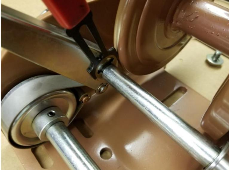
8. Next, snap retaining ring (KK) back onto drive shaft in front of Brake Handle Assy (X) using snap-ring pliers or a retaining ring applicator. The intermediate drive shaft should now be fully locked into place, and should have adequate gear mesh with the primary drive shaft (EE).
