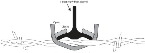
Position Grip on wire and post. Crimp closed to lock in place.
